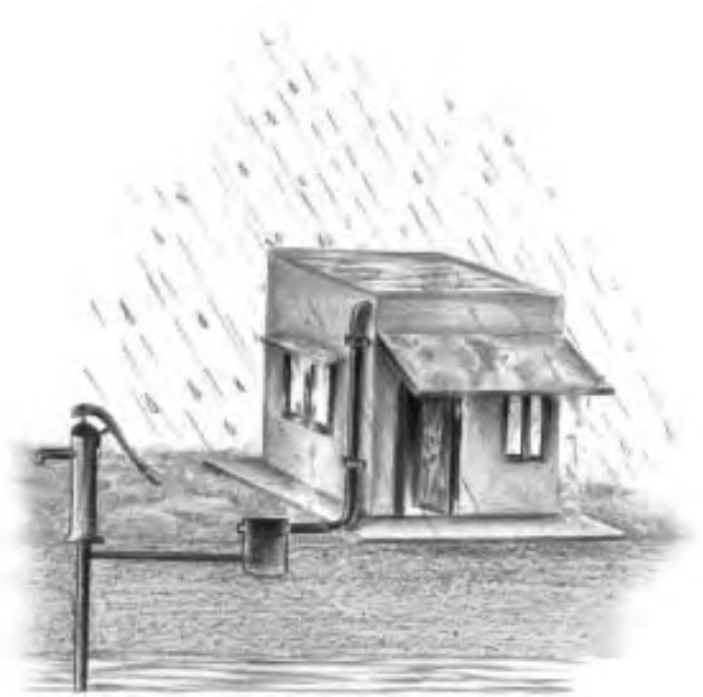
(a) Recharge through Hand Pump
