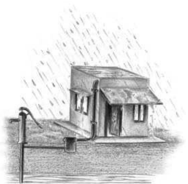
(a) Recharge through Hand Pump
